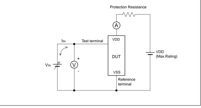
Note : The voltage V<sub>IN</sub> is increased gradually and the current I<sub>IN</sub> of 300 mA at maximum shall flow. Confirm the latch up does not occur under I<sub>IN</sub> =  $\pm$  300 mA.
