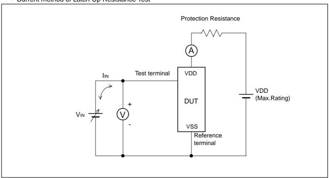
Note: The voltage  $V_{IN}$  is increased gradually and the current  $I_{IN}$  of 300 mA at maximum shall flow. Confirm the latch up does not occur under  $I_{IN}=\pm300$  mA. In case the specific requirement is specified for I/O and  $I_{IN}$  cannot be 300 mA, the voltage shall be
