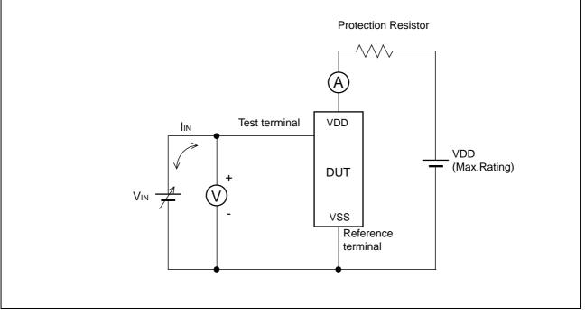
Note : The voltage V<sub>IN</sub> is increased gradually and the current I<sub>IN</sub> of 300 mA at maximum shall flow. Confirm the latch up does not occur under I<sub>IN</sub> = ± 300 mA. In case the specific requirement is specified for I/O and I<sub>IN</sub> cannot be 300 mA, the voltage shall be increased to the level that meets the specific requirement.
