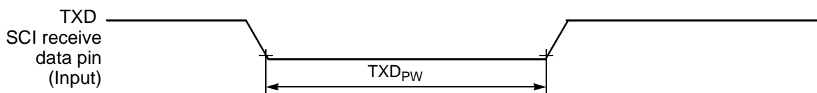
Figure 27. TXD Pulse Width
