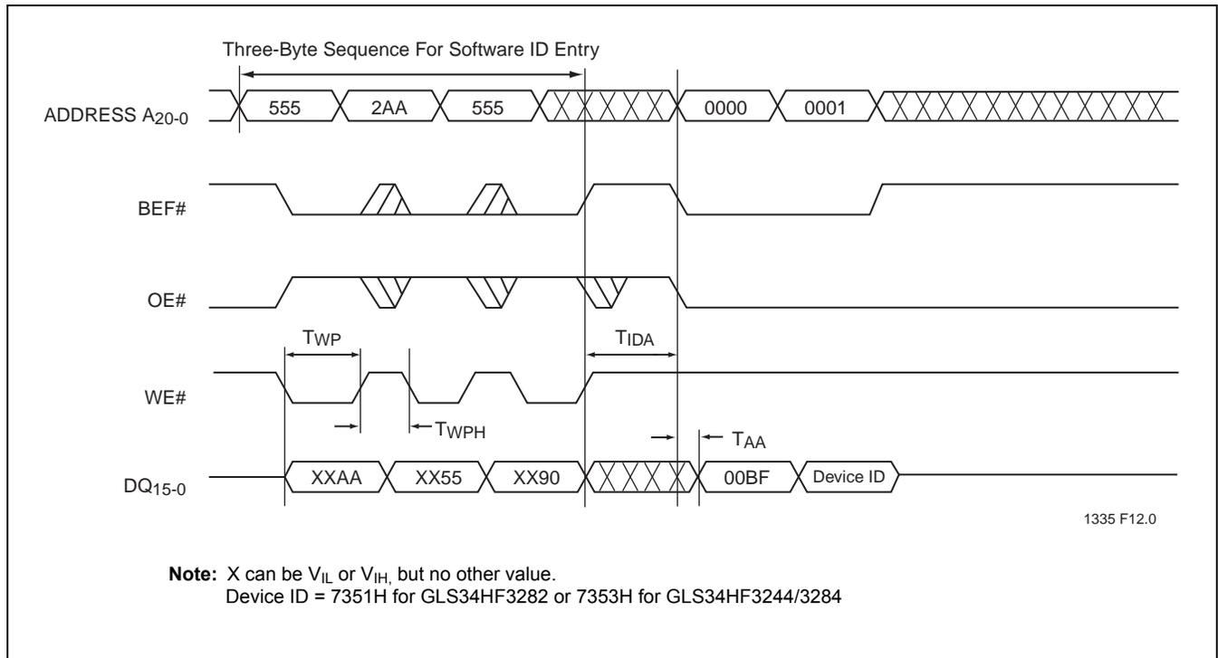
FIGURE 15: Flash Software ID Entry and Read (For Byte Mode A<sub>1</sub> = 0)
