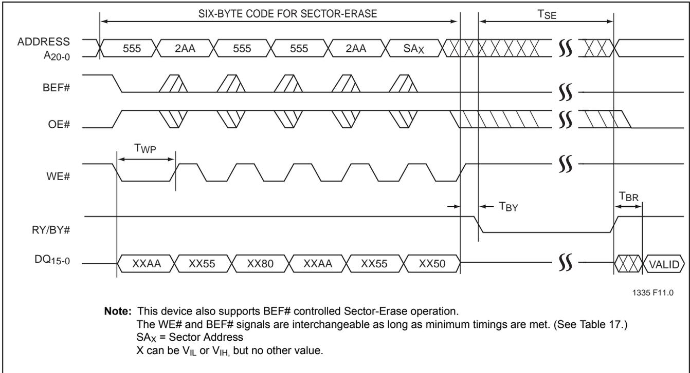
**FIGURE 14: Flash WE# Controlled Sector-Erase Timing Diagram for Word Mode
