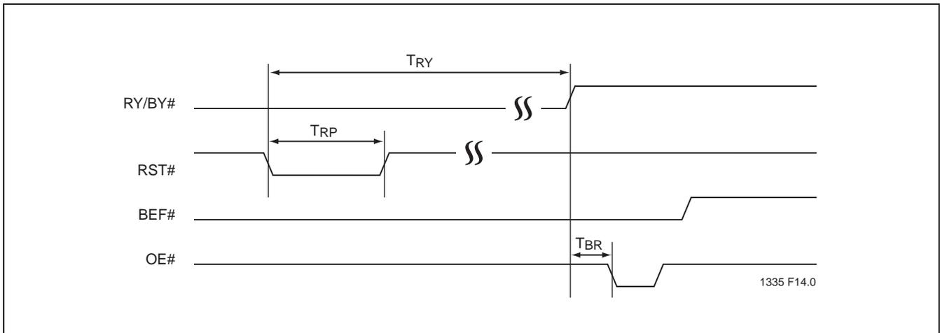
**FIGURE 19: RST# Timing (during Sector- or Block-Erase operation)**
