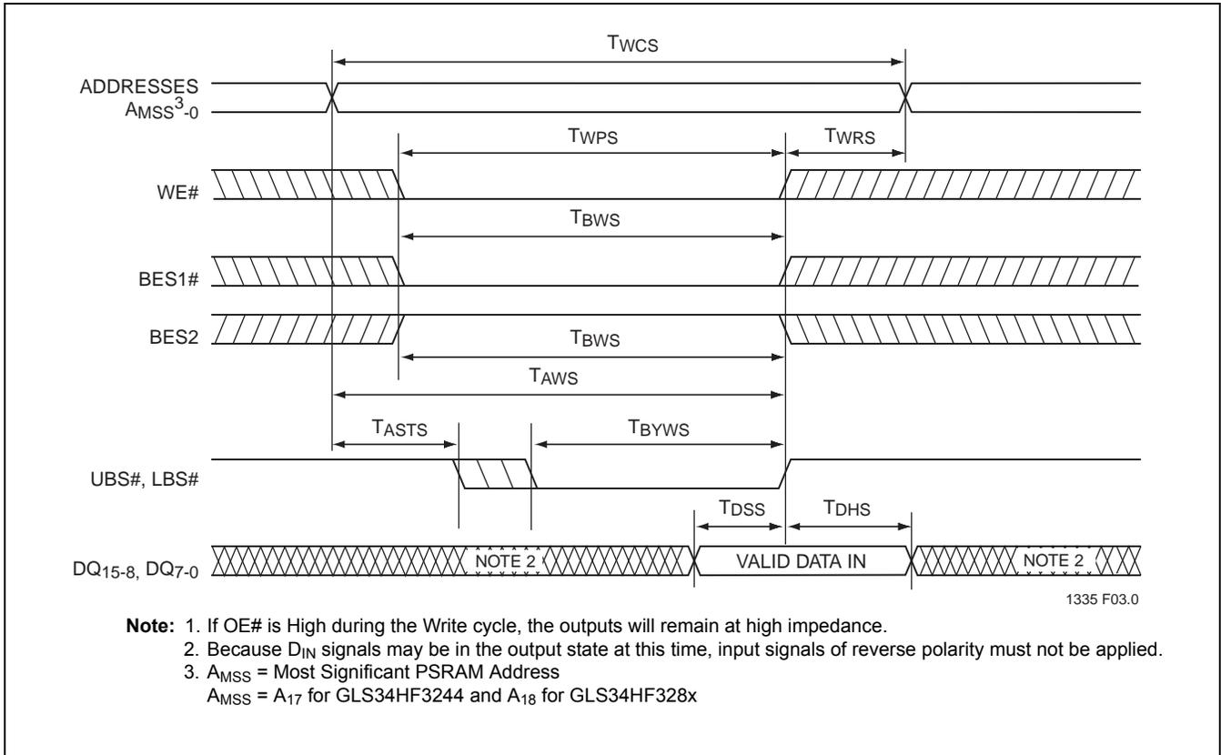
FIGURE 6: PSRAM Write Cycle Timing Diagram (UBS#, LBS# Controlled)<sup>1</sup>
