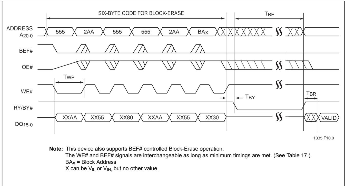
**FIGURE 13: Flash WE# Controlled Block-Erase Timing Diagram for Word Mode
