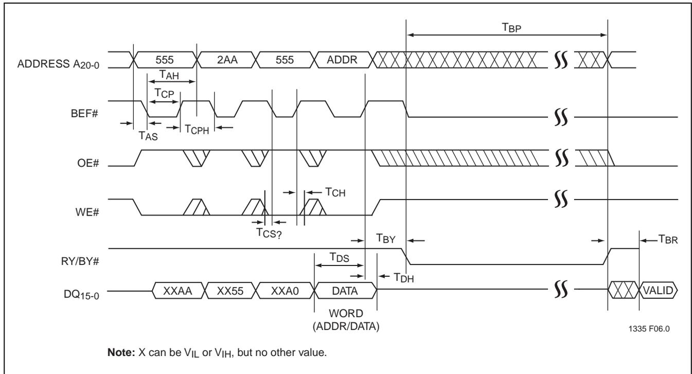
**FIGURE 9: Flash BEF# Controlled Program Cycle Timing Diagram for Word Mode
