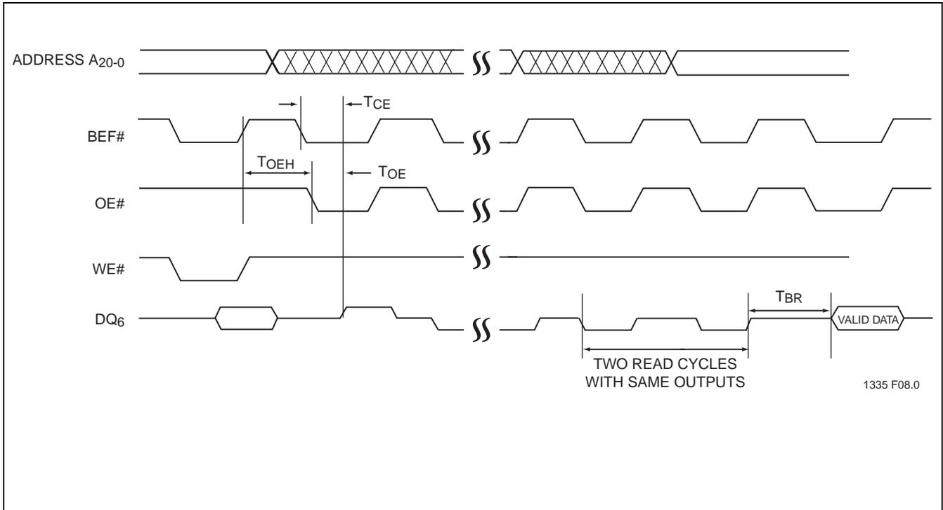
**FIGURE 11: Flash Toggle Bit Timing Diagram for Word Mode
