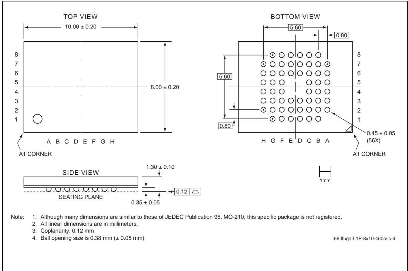
**FIGURE 27: 56-ball Low-profile, Fine-pitch Ball Grid Array (LFBGA) 8mm x 10mm
