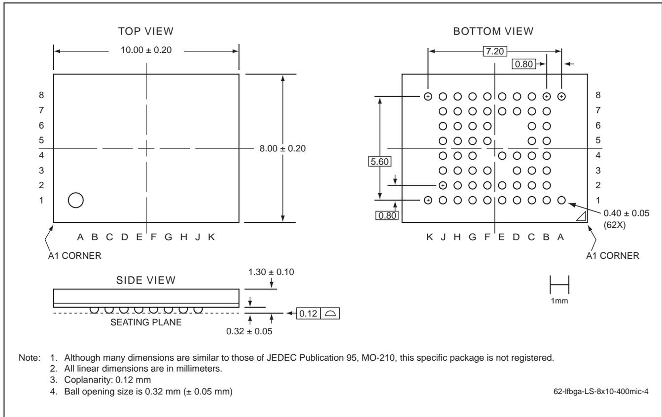
**FIGURE 28: 62-ball Low-profile, Fine-pitch Ball Grid Array (LFBGA) 8mm x 10mm
