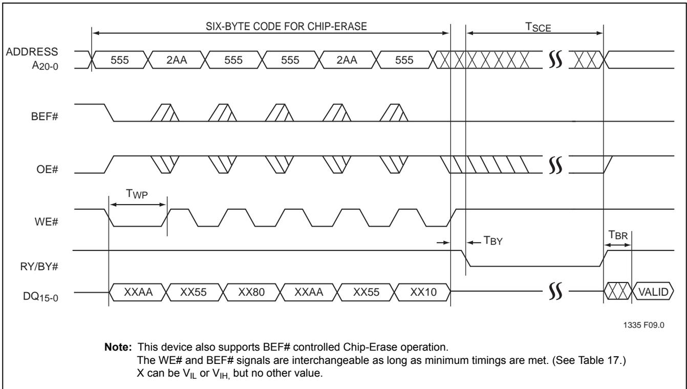
**FIGURE 12: Flash WE# Controlled Chip-Erase Timing Diagram for Word Mode
