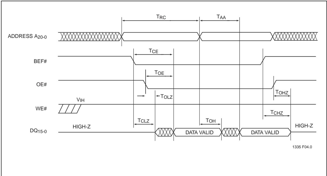
**FIGURE 7: Flash Read Cycle Timing Diagram for Word Mode
