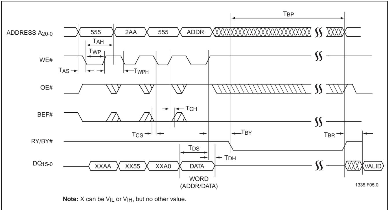
**FIGURE 8: Flash WE# Controlled Program Cycle Timing Diagram for Word Mode
