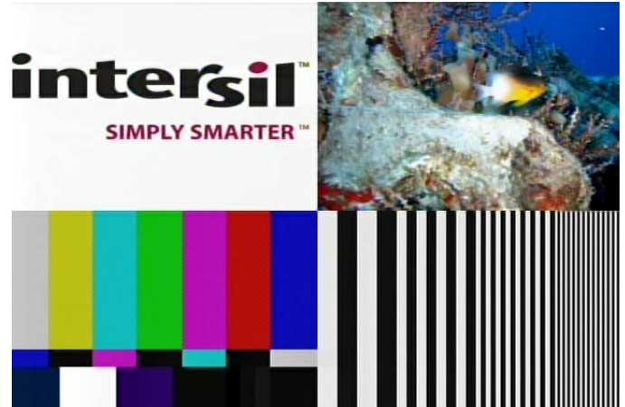
FIGURE 2. TEST PATTERN IMAGE AFTER 1000 FEET OF CAT 5 WITH ISL59601 (OR BETTER)
