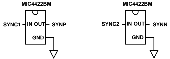
FIGURE 22B. NON-INVERTING DRIVERS
