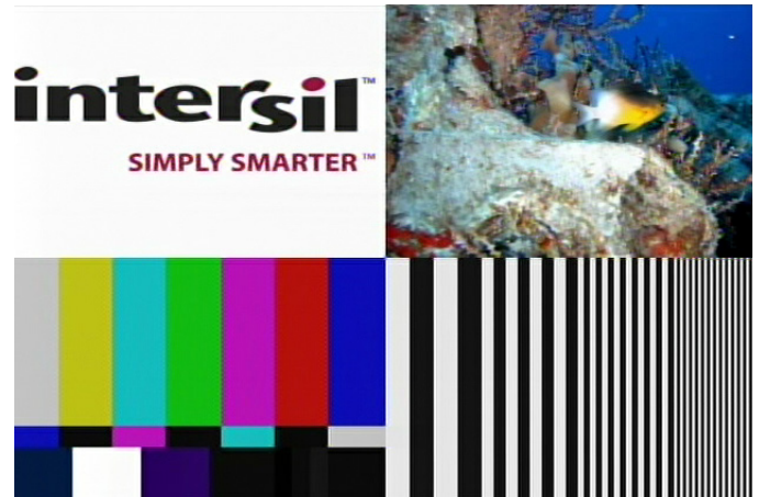
FIGURE 22. TEST PATTERN IMAGE AFTER 1000 FEET OF RG-59 COAX WITH ISL59601 (OR BETTER)
