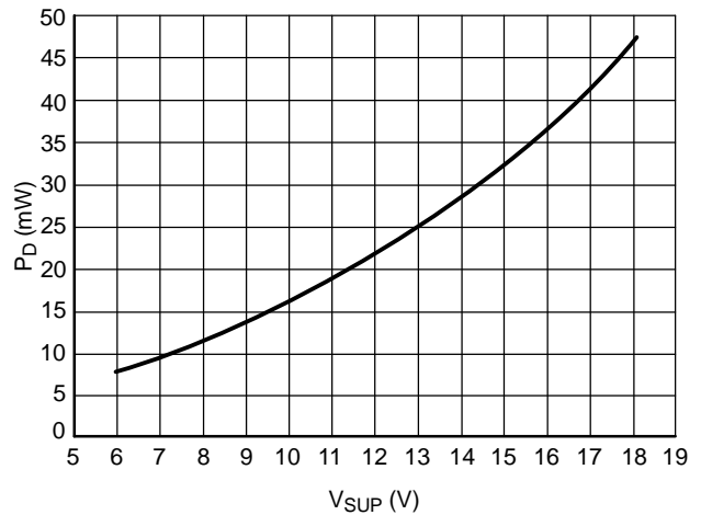
Figure 28. Power Dissipation LIN Transceiver @ 20 kbit
