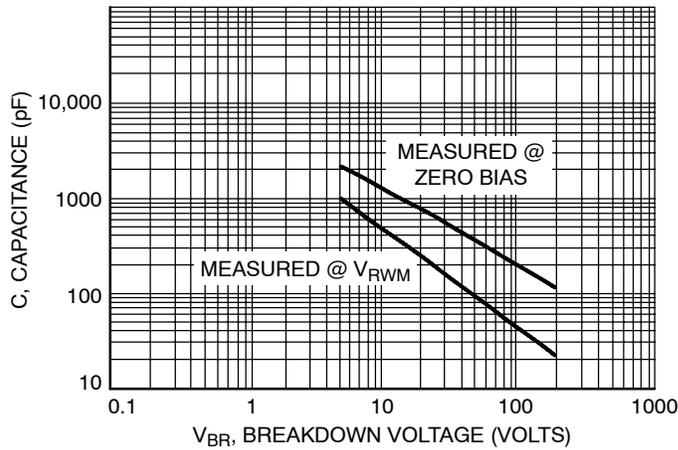
Figure 4. Capacitance versus Breakdown Voltage
