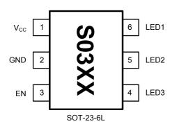
NOTE: The location of pin 1 on the S03XX is determined by orienting the package marking as shown.
