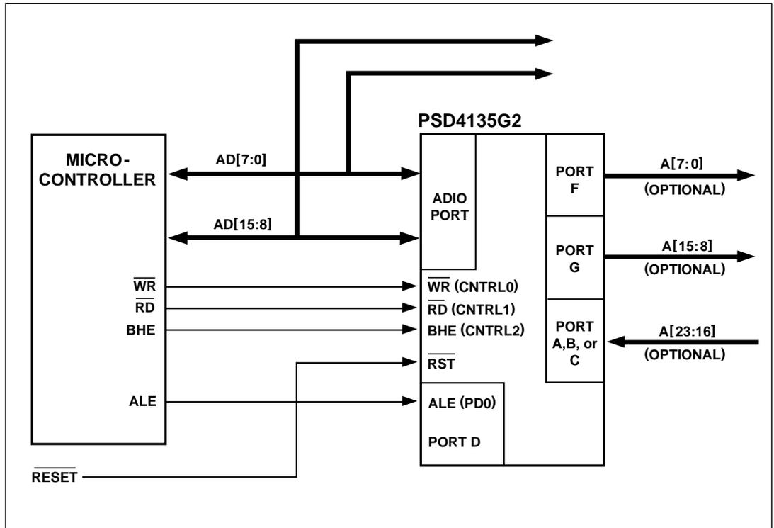
Figure 13. An Example of a Typical 16-Bit Non-Multiplexed Bus Interface
