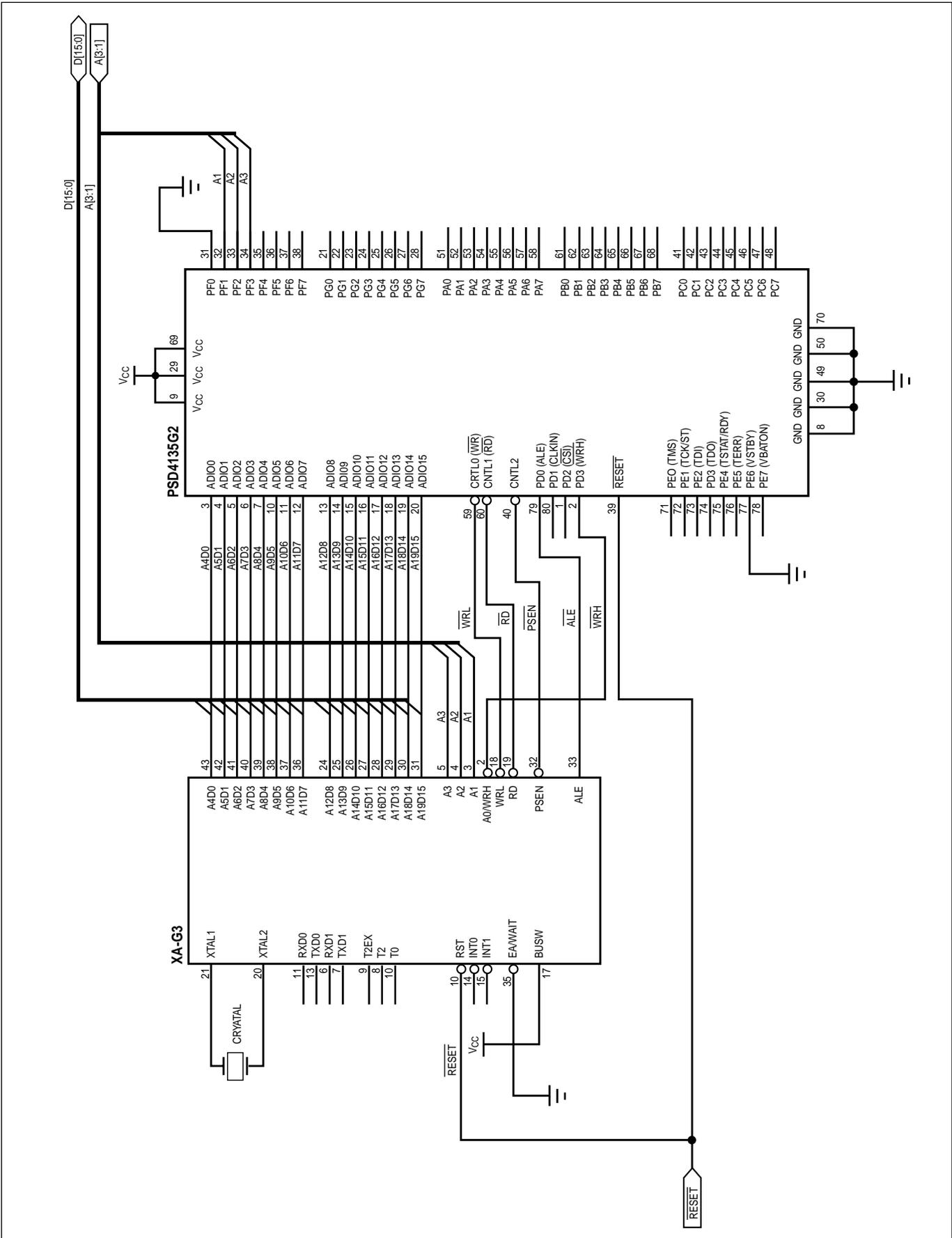
Figure 18. Interfacing a PSD4135G2 with a MMC2001
