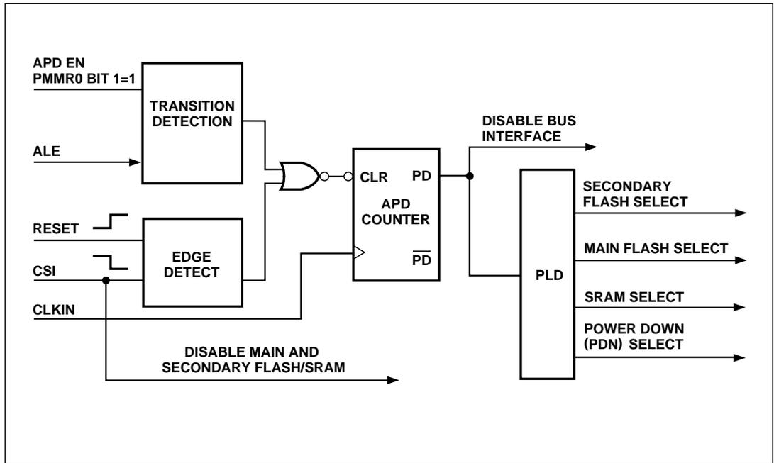
Figure 25. Enable Power Down Flow Chart
