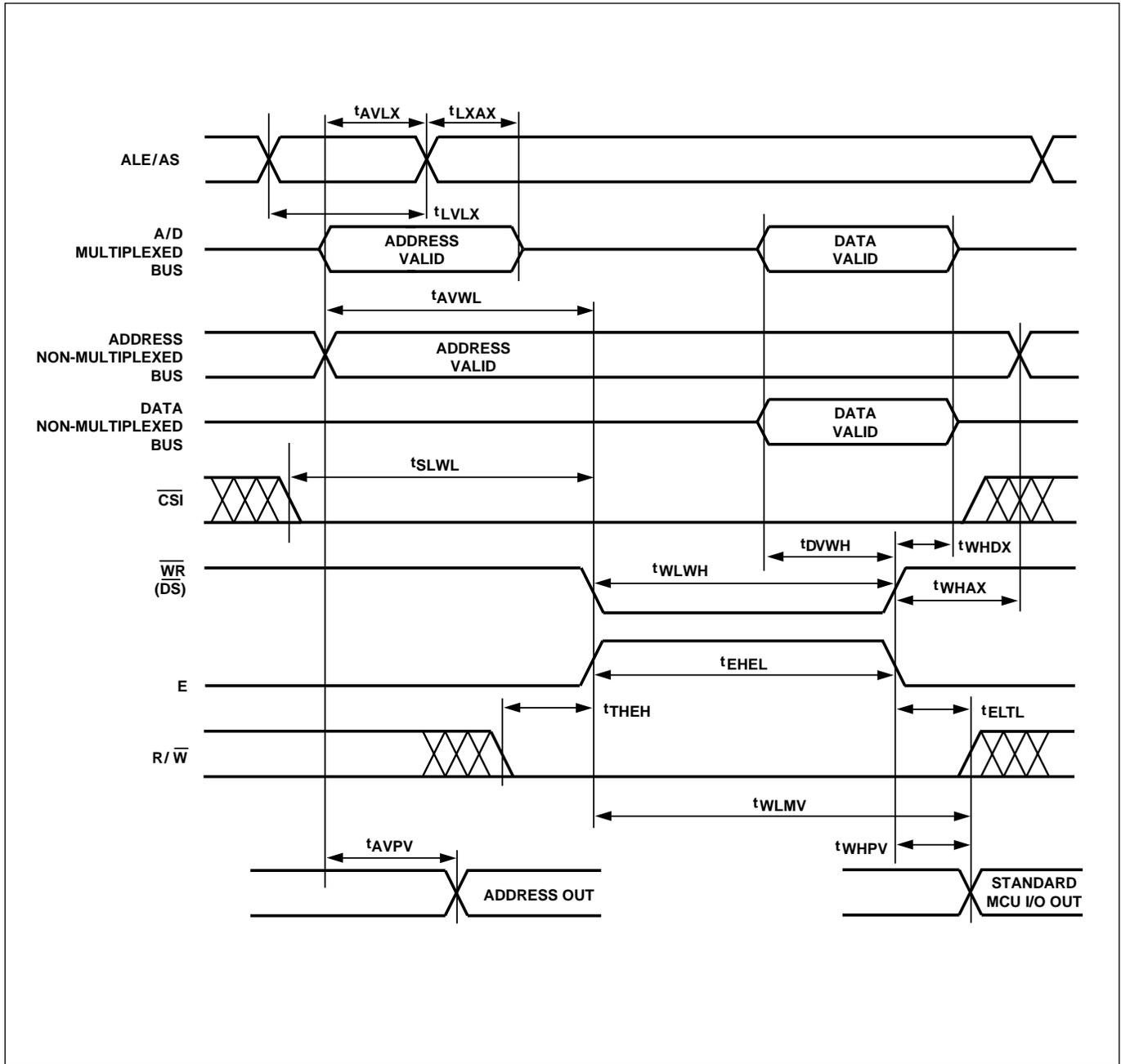
Figure 30. Combinatorial Timing - PLD
