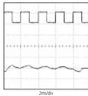
LINE-TRANSIENT RESPONSE ( I_{OUT} = 20\text{mA} )
